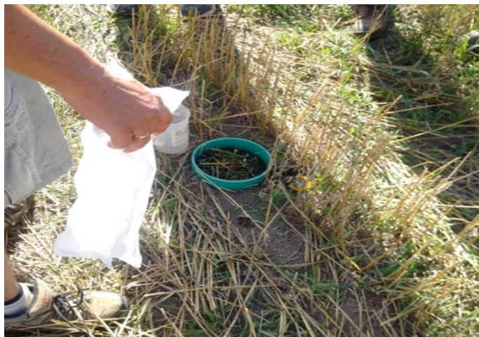
Figure 1. Water Infiltration test. A measure of the amount of time it takes rainfall to infiltrate into the soil. It is measured by pouring 1" of water in an 8" ring and recording amount of time it takes for water to soak into the soil.
