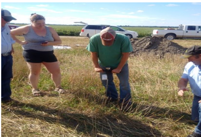
Figure 2. Hands-on demonstration of using a penetrometer to measure surface hardness in the top 0" to 18" (measured in psi), conducted at the Field Day August 29 th . The penetrometer or tile probe can be used to confirm the areas of the field where soil compaction exist. In some cases, such as this field, the soil is too dry to measure. Ensure the soil is moist (i.e. 2 days after a good rain).
